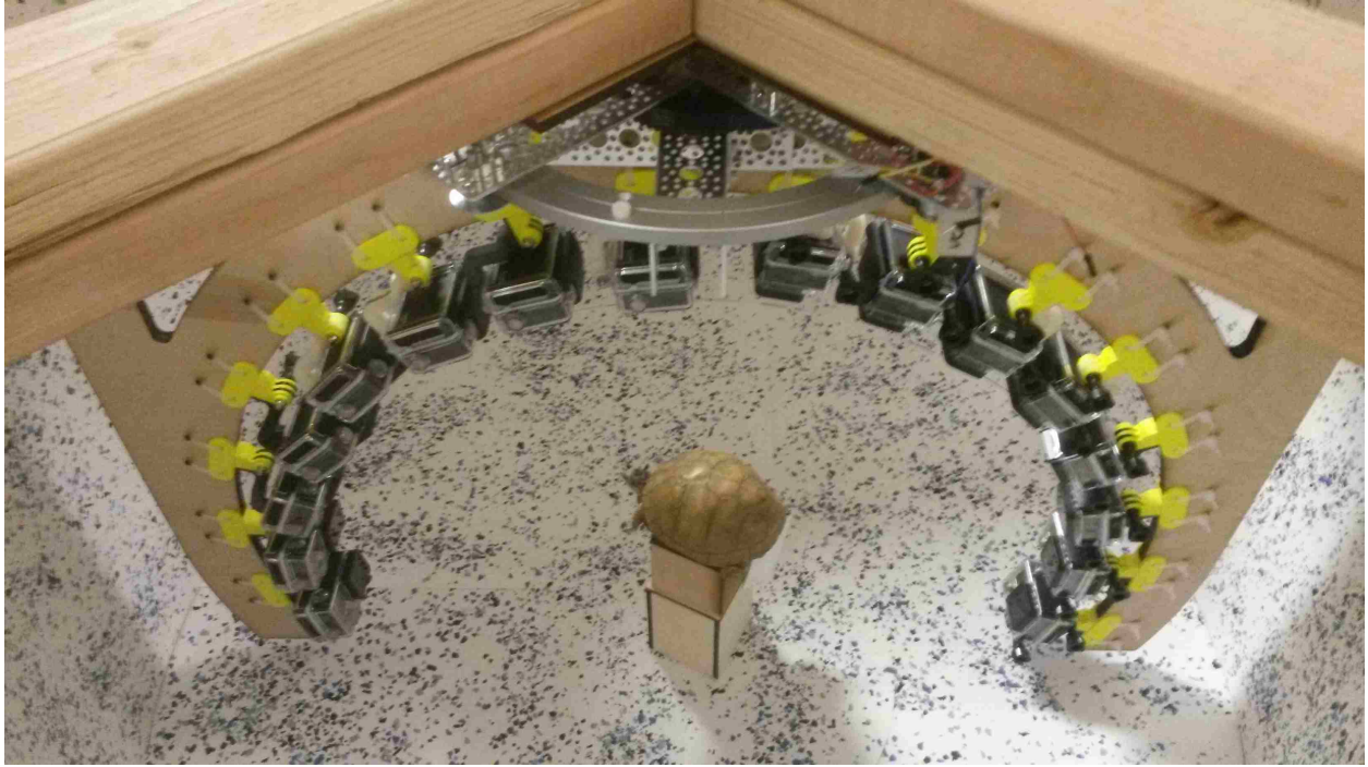
Figure 3.1: Arch containing 16 cameras
